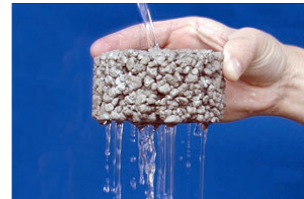
Permeable surfaces can be used when both a durable surface and infiltration is needed.
